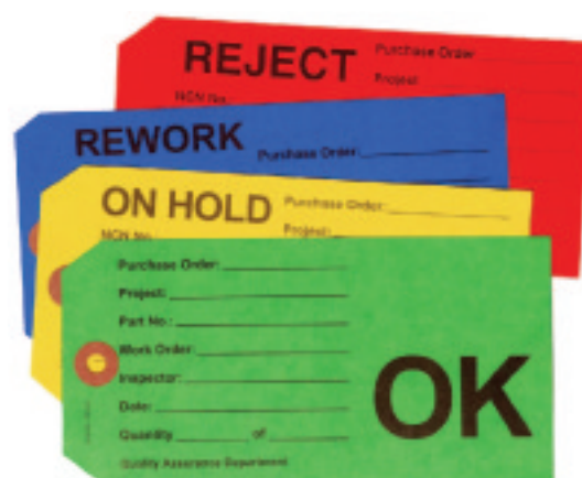
Rework is one of the seven wastes in traditional lean manufacturing terms and requires excessive, manual interception and robust quality control systems, as these quality control tags used in manufacturing environments demonstrate.
